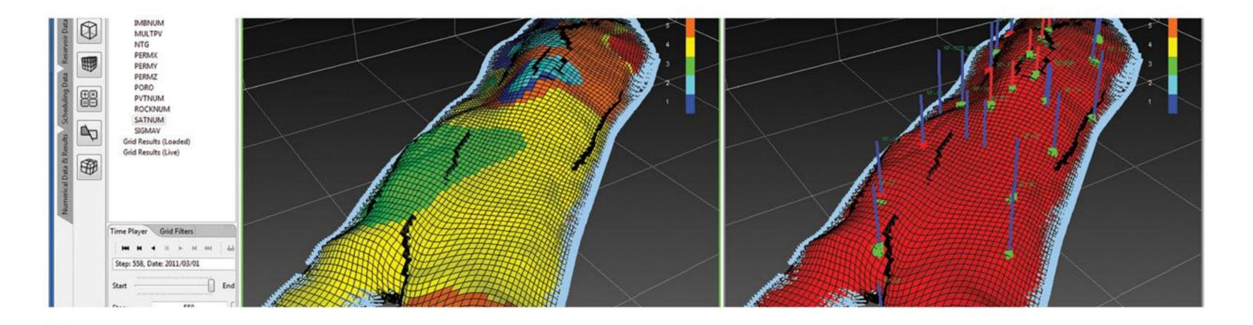
Single well simulation using explicit DFN model to predict the well performance. The results of this simulation are usually used to design the Hydraulic Fracturing operation and predict the future performance of wells. An overall skin factor is also estimated for full field studies.
