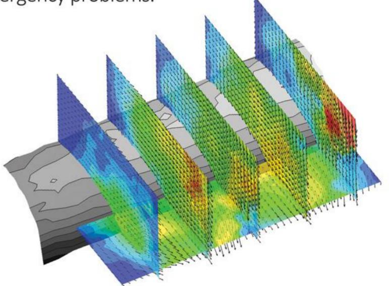
The AMG technology is one of the most recent strategies for solving matrices generated in elliptic partial differential equations that can produce suitable solutions for complicated problems.
